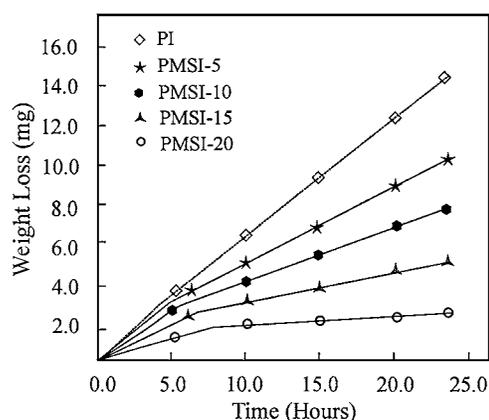
Figure 3 Weight loss versus exposure time in the oxygen plasma asher for polyimide and PMSI blends.
