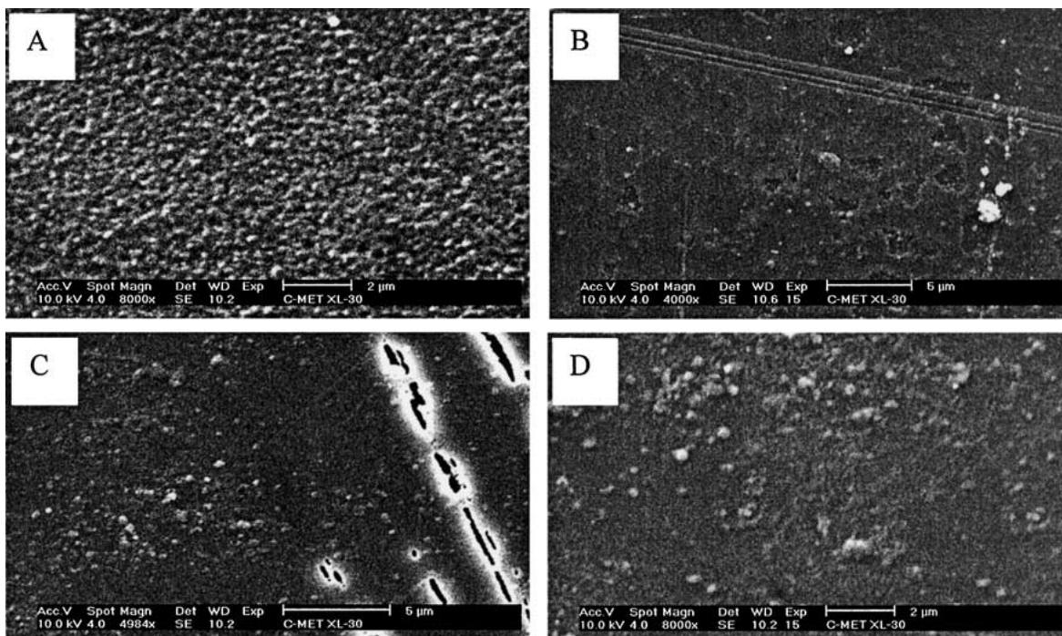
Figure 4 SEM of oxygen plasma exposed neat polyimide (A), PMSI-5 showing surface erosion (B), PMSI-10 showing oxidized silica particles and cavitation on surface (C), PMSI-20 showing dispersed silica particles and unaffected surface (D).
